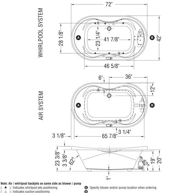
( • ): Indicates airjets positioning ( ): Indicates standard grab bar positioning (  $\frac{\Psi}{\Box}$  ): Indicates chromatherapy light positioning Bathtub base includes anti-vibration Neutra-Phone leg supports (not shown).
