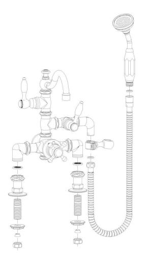
This faucet is tested to remain within 1 degree Fahrenheit of your desired setting throughout its operation, with an automatic temperature stop at 104 degrees Fahrenheit. The unit also has a built-in anti-syphon.
